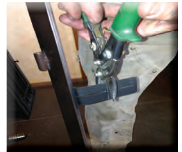
6. Trim the welded tabs, if needed to the measured length..
